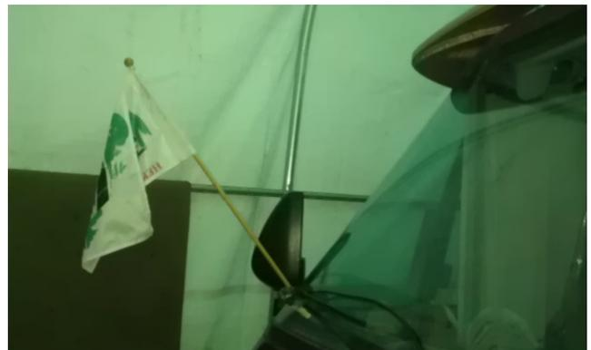
Here is a simple flag holder made from a chrome shower pipe and painted black. Drill one hole and use a bolt from the mirror to mount the flag holder. A wooden dowel is used as the flag pole.
